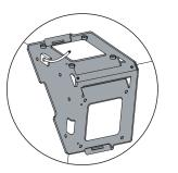
Jamb Drill for cable 0.5 in (12 mm from top of the system and 3.5 in (89 mm) from back of the system.
