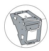
Ceiling Drill for cable 2.5 to 4.5 in (64 to 114 mm) from back of the system and 1.5 to 3.75 in (38 to 95 mm) from end of the system.
